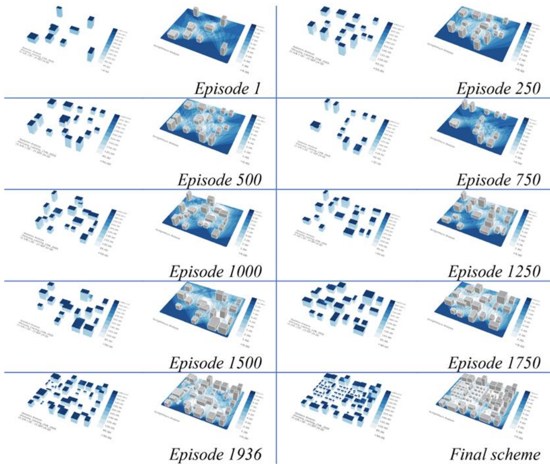
Figure 3.6 Sample of the sequential generation process of an urban block by a DRL agent. (Reprinted from Han et al., 2021, p.141)
