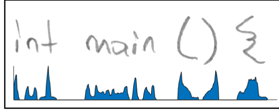
Figure 3.9 Vertical histogram projection of a text line
