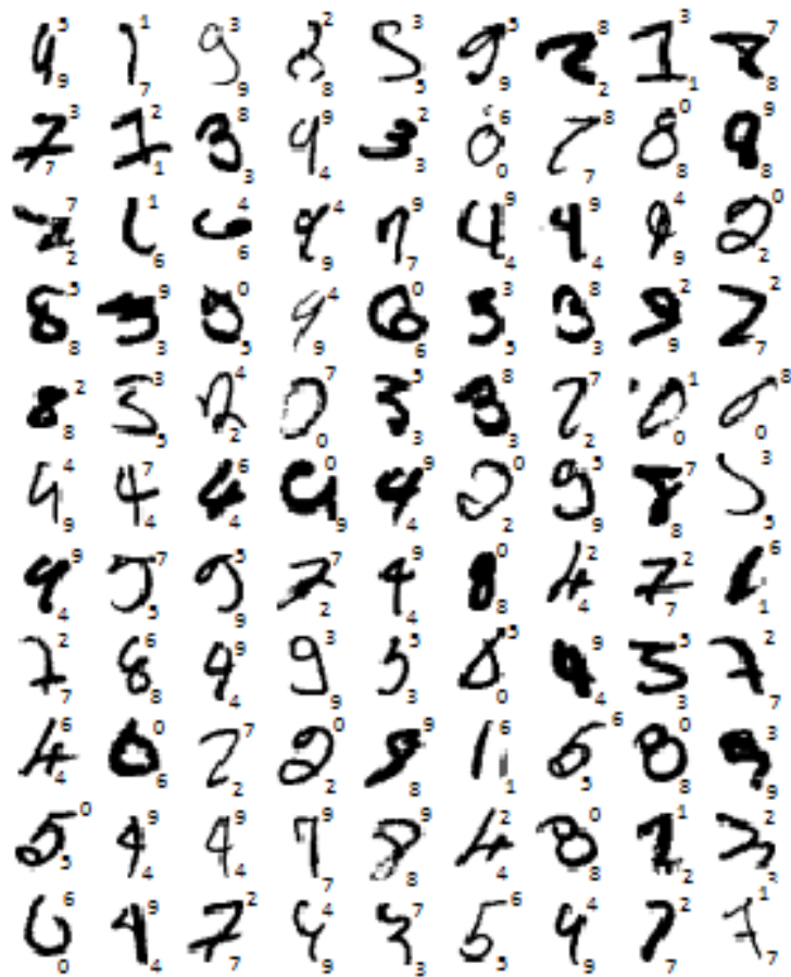
Figure 4.19: The 99 misclassified test cases for the given confusion matrix in Table 4.8 where subscript represents the expected label and superscript represents the network's guess
