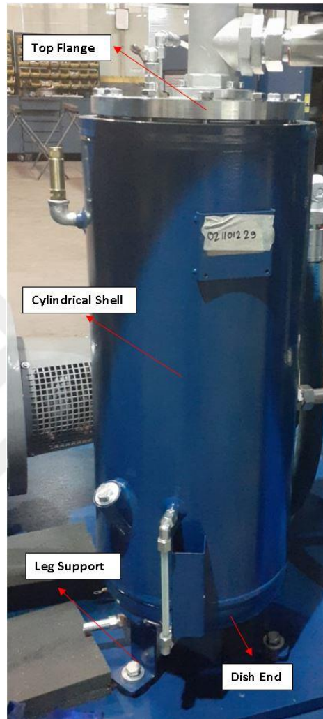
Figure 3.1. Figure of in-house developed oil separator pressure vessel components.
