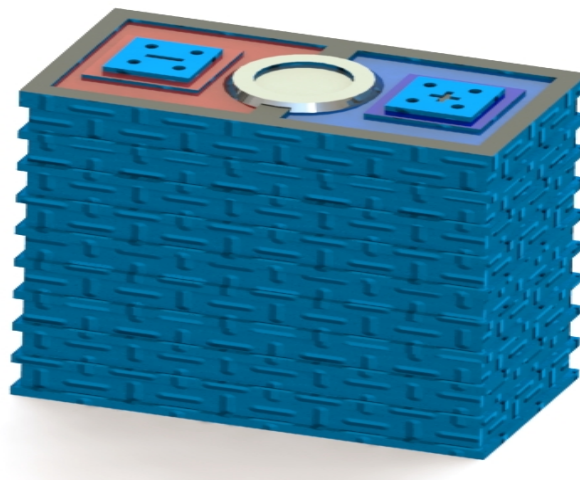
Figure 3.15. Designed battery module
