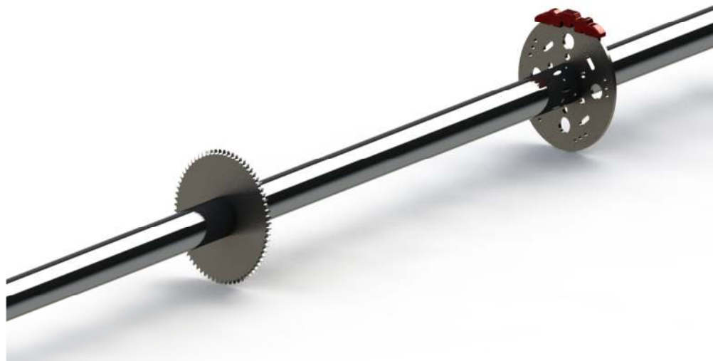
Figure 3.21. Design of the rear axle including brake pad and gear wheel
