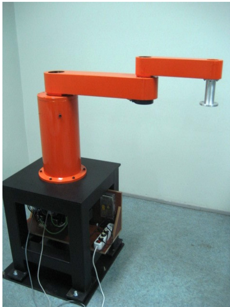
Figure 3.34 Assembled SCARA robot and console system
