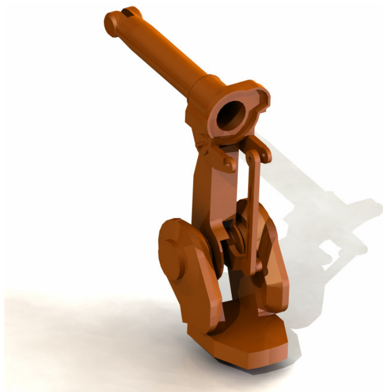
Figure 4.2 The solid CAD model of the ABB IRB 1400
