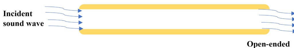
Figure 5.4: Schematic diagram of hollow glass fibre
