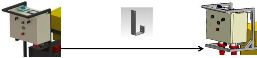
Figure 5.10 Panel vibration solution
