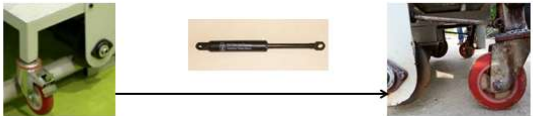
Figure 5.18 Caster with gas spring
