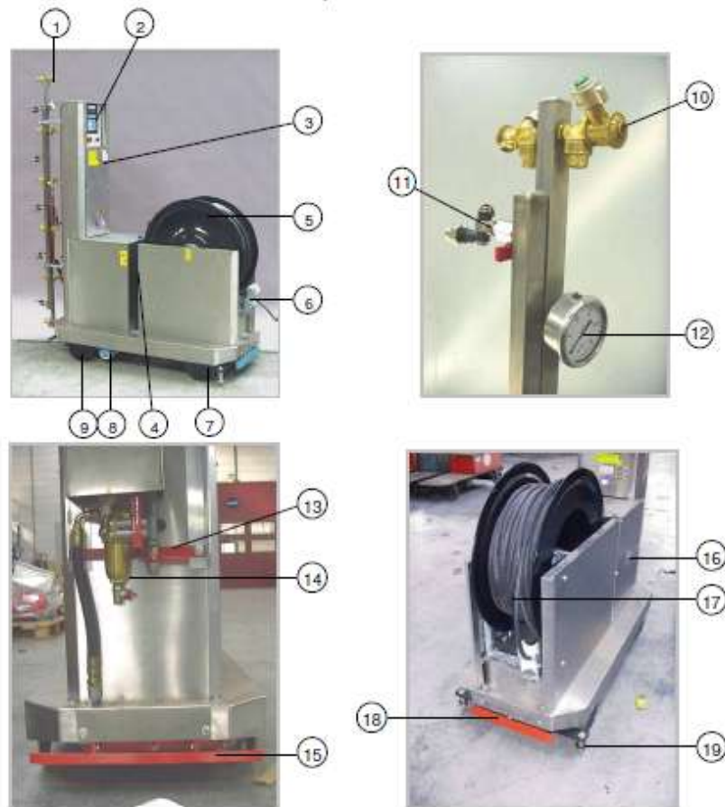
Figure 1.6 Main part of the spray trolley (IDM Product)
