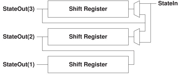
Figure 3.19 Block diagram of the memory unit of a Falcon processor [6]
