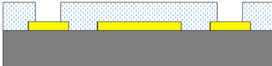
(b) After the deposition and the patterning of the sacrificial layer.
