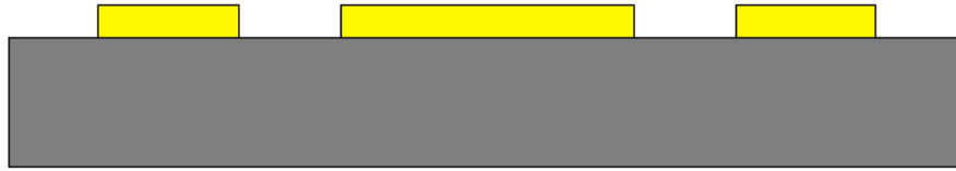
(a) After the deposition and the patterning of the mirror layer and the connection pads.
