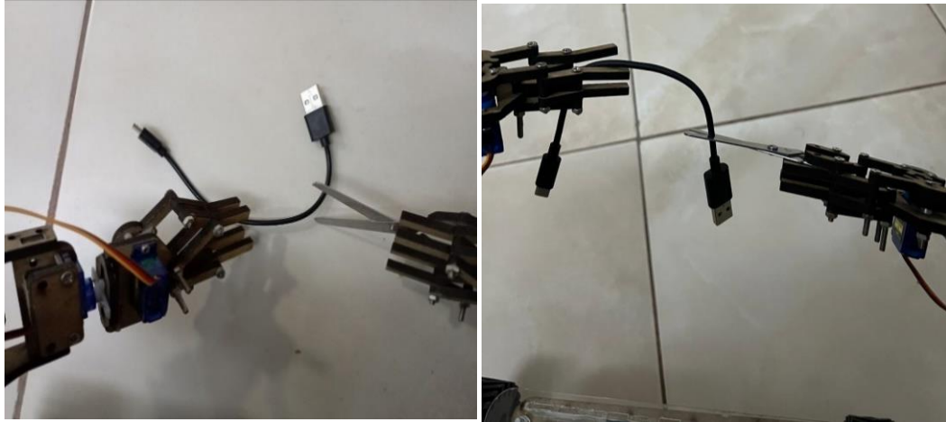
Figure 4.6 Testing for cutting and holding a short cord for a phone charger with the help of a camera
