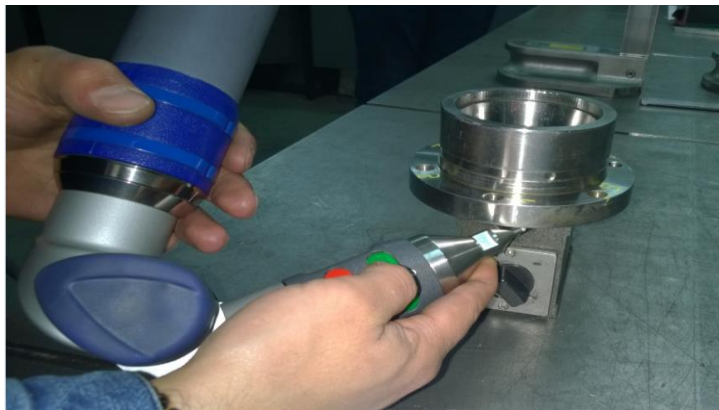
Figure 5.20: 3-D Quality Control of Housing
