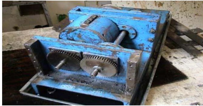
Figure 2.11: A Power Circulation Test Rig Designed by Sachidananda, Gonsalvis, Prakash and Rajesh
