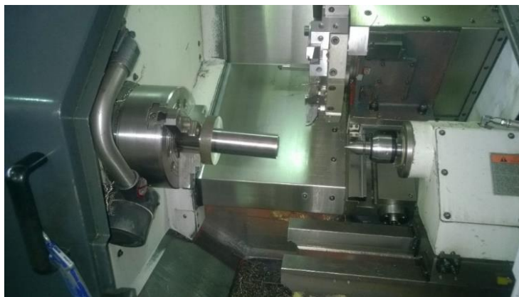
Figure 5.3: Fine Turning of Shaft with CNC Turning Machine
