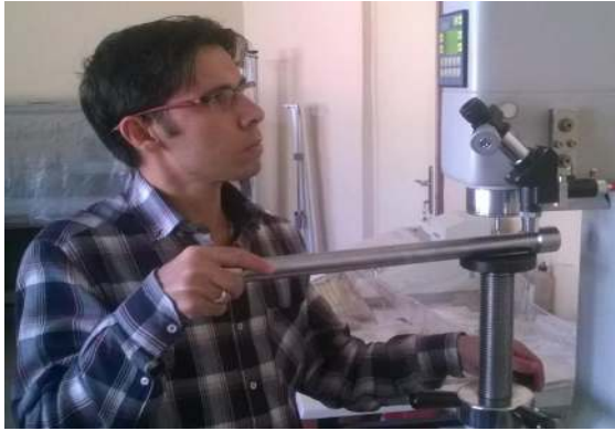
Figure 5.19: Hardness Test Of Rod
