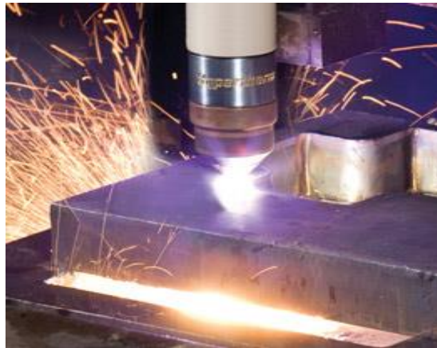
Figure 5.8: Plasma Cutting of Gear Box Components
