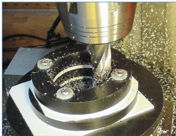
Figure 5.6: Milling Process of Couplings
