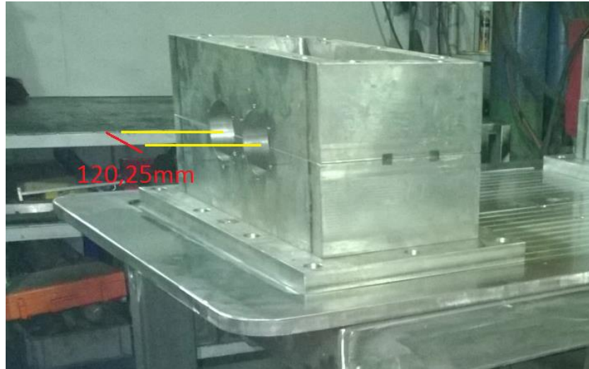
Figure 4.58: Center Distance of Gears after Production
