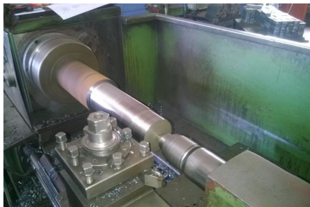
Figure 5.2: Rough Turning of Shaft with Universal Turning Machine
