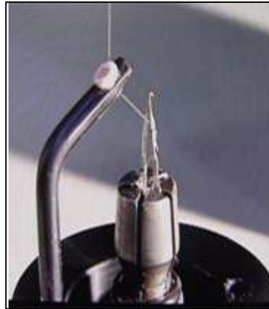
Figure 4.1: A Narrow Circular Knitting mechanism with five needles. The thread guide is delivering yarn into the needle hooks as it rotates about the needles.
