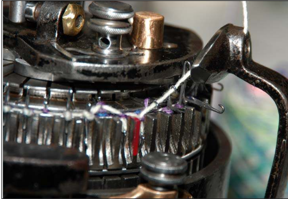
Figure 3.5: Cylindrical needle bed of a circular knitting machine. The thread guide is seen delivering the thread to the hooks of the needles.
