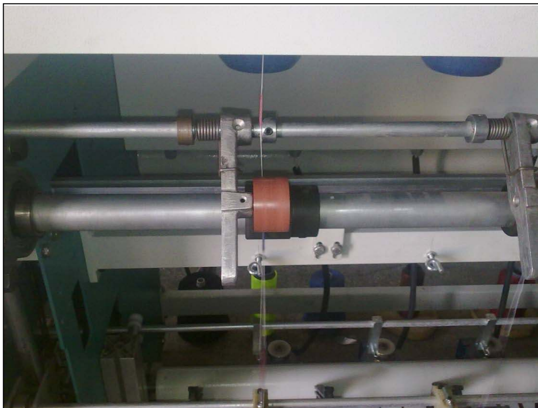
Figure 6.3: The bottom half of the frontal view of the prototype fancy yarn machine, showing the yarn advancing and winding system.
