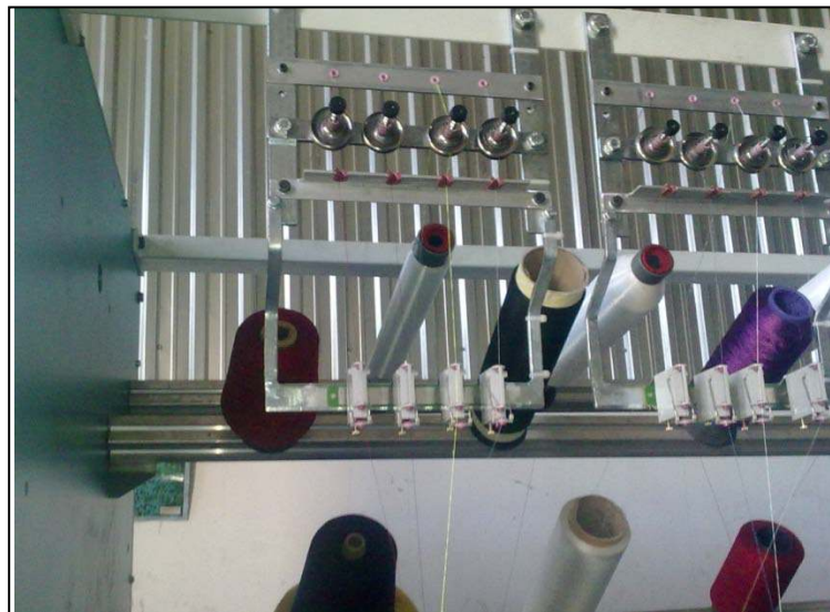
Figure 6.2: The back side view of the prototype fancy yarn machine showing the creel, yarn tensioning devices and yarn rupture detectors.
