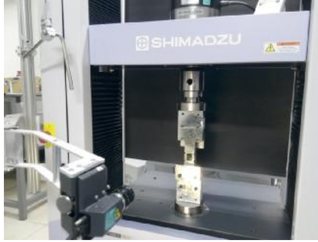
Figure 4.16. Compressive test specimen under compression load.
