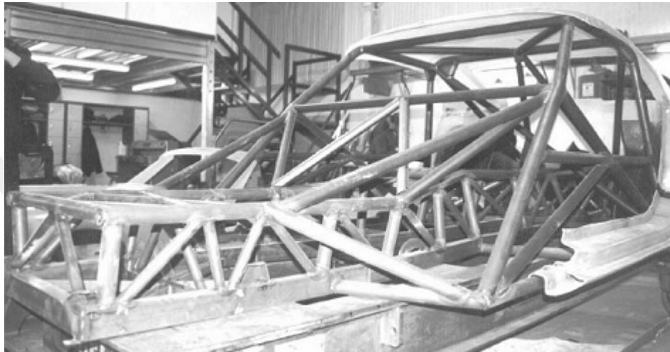
Figure 3.12. Triangulated sports car structure with integrated roll cage.
