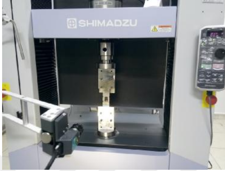
Figure 4.24. A standard open-hole compressive test specimen under compression load.
