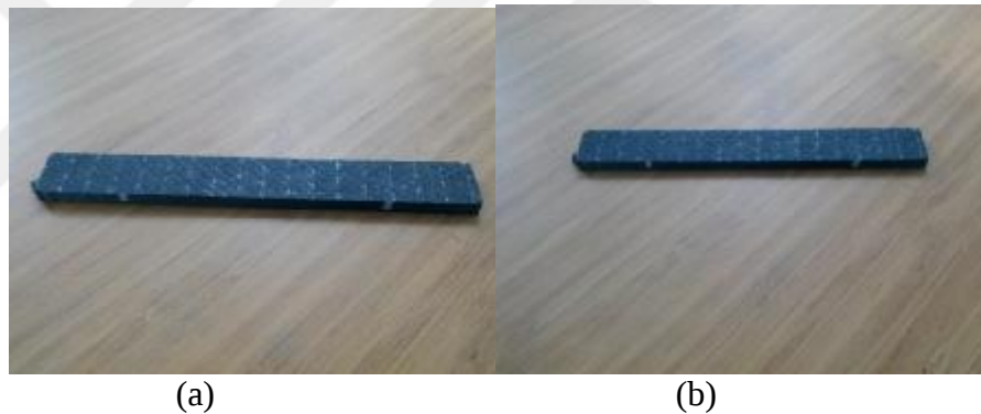
Figure 4.11. Flexural test specimens (a)the specimen in 0^\circ direction,(b)the specimen in 90^\circ direction.
