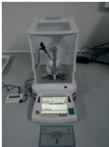
Figure 4.4. Weighing by means of a pair of scales of the specimen
