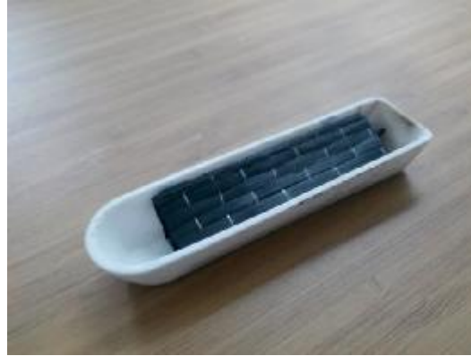
Figure 4.6. Unidirectional carbon fiber fabric in a porcelain crucible after burning off.
