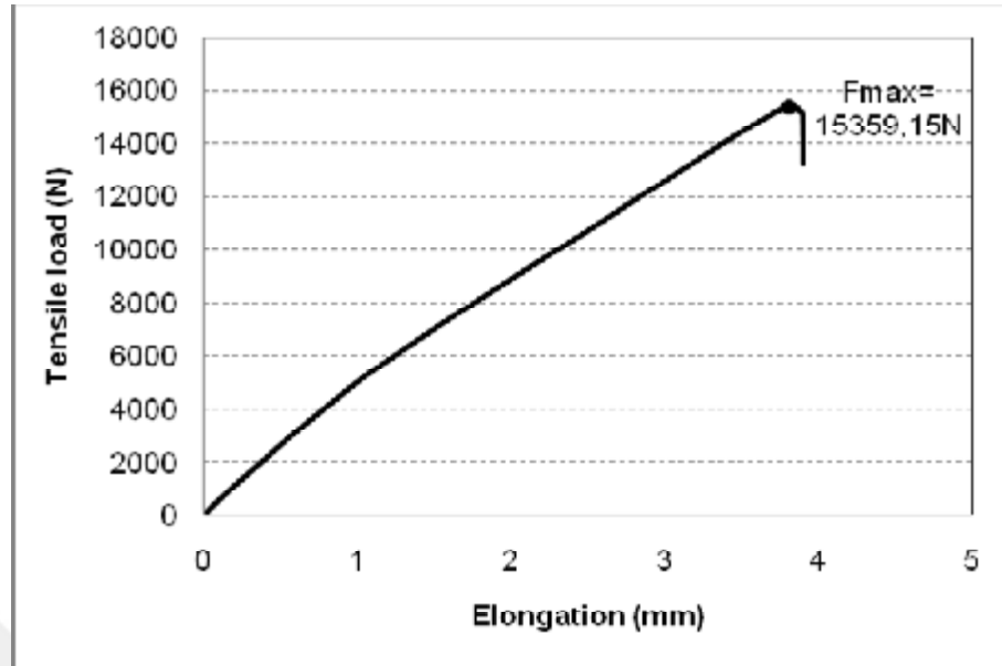
Figure 4.9. Typical load-elongation curve of a unidirectional [0]_4 carbon/epoxy specimen under static tensile loading.
