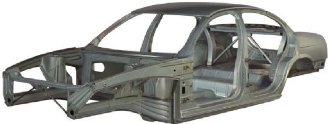
Figure 3.18. Modern integral body in white.
