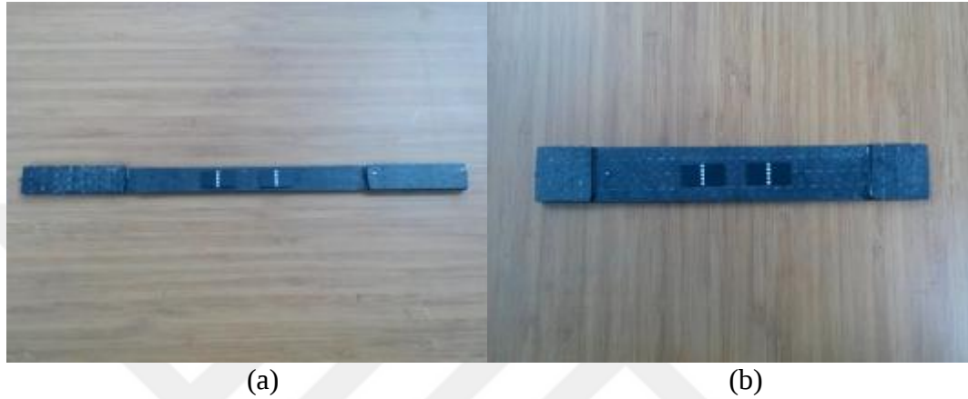
Figure 4.7. Tensile test specimens (a)the specimen in 0^\circ direction,(b)the specimen in 90^\circ direction.
