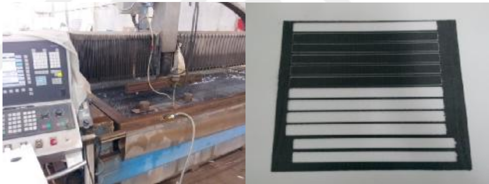
Figure 4.2. Cutting the specimens with the help of CNC water jet cutting machine as required by the ASTM standard test methods.
