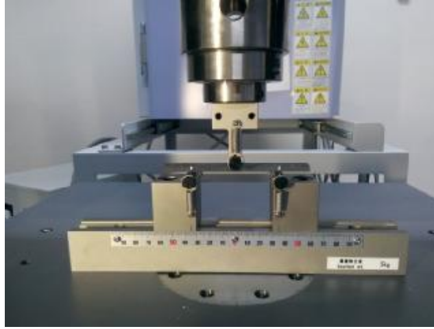
Figure 4.12. Flexural test specimen during test
