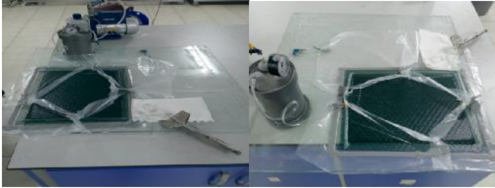
Figure 4.1. Preparation laminated composite material samples with the aid of a vacuum infusion techniques.
