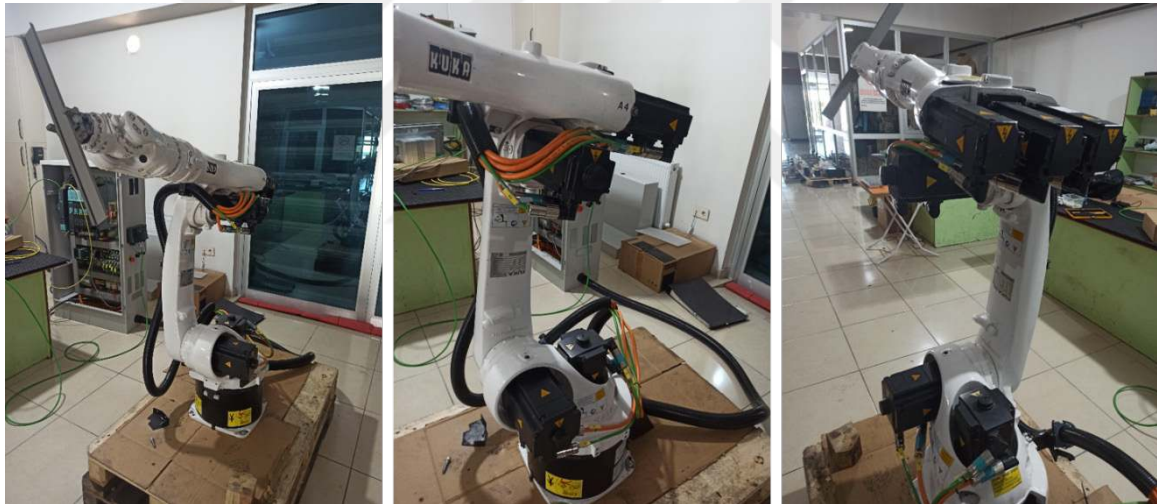
Figure 4.8. KUKA KR-5 ARC-C Robot with Motors Mounted
