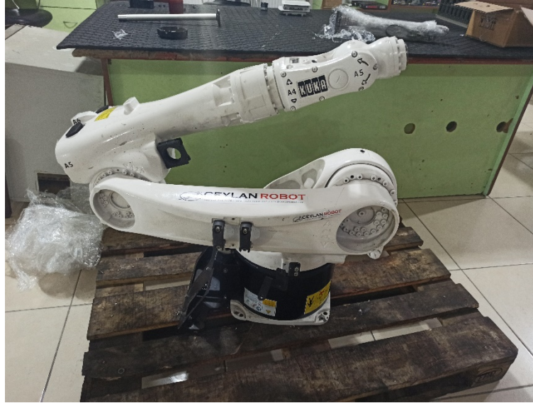
Figure 1.4. An Industrial Robotic Arm KUKA KR5 ARC-C With no Electronic Components
