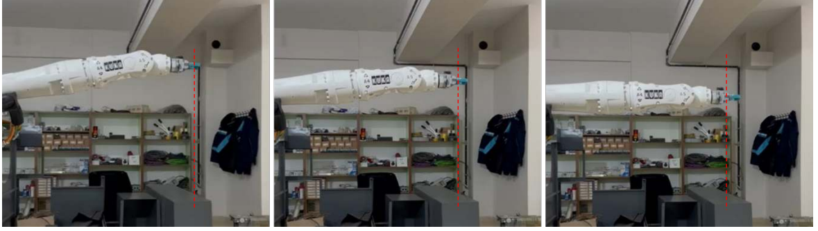
Figure 5.19. Physical Test of KUKA KR5 for the Linear Motion Along the Z-Axis
