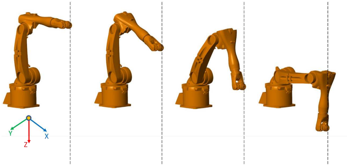
Figure 5.13. KUKA KR5 Visual Simulation for the Linear Motion Along the Z-Axis
