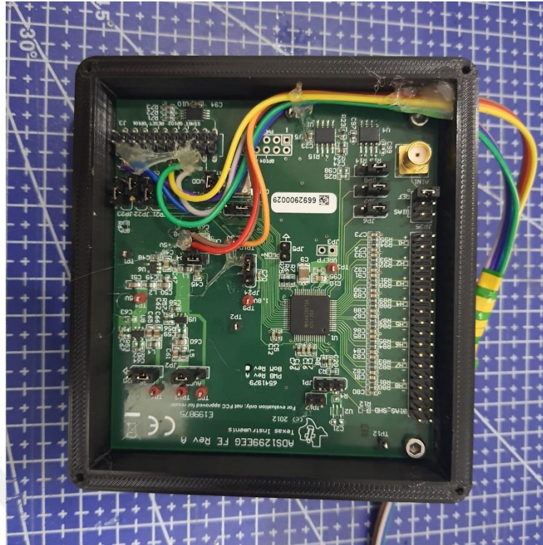
Figure 3.2 Texas Instruments ADS1299EEGFE-PDK Performance Development Kit used in Project
