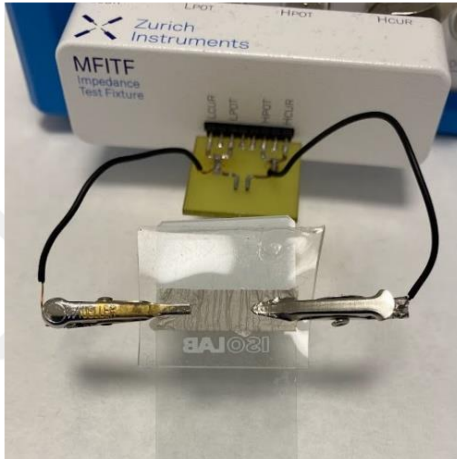
Figure 2.4: Characterization of the sensor without encapsulation and cabling.
