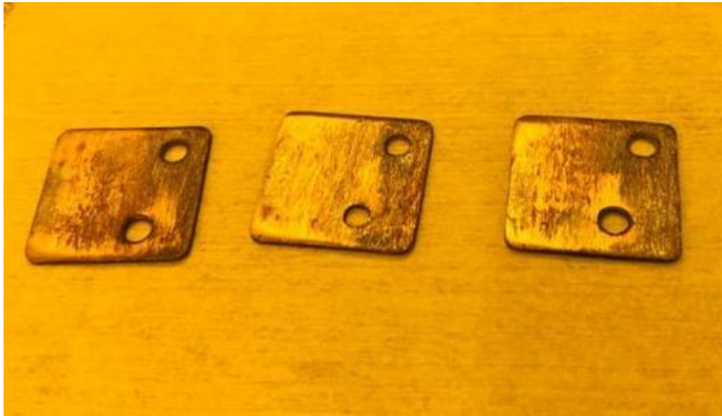
Figure 3-3. Cleaned copper plates for the laser bonding
