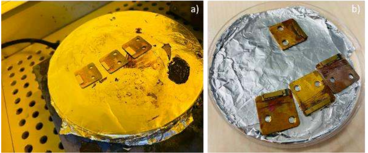
Figure 3-8. a) The view of laser bar's on the hot plate, b) the image of ready bar's to test
