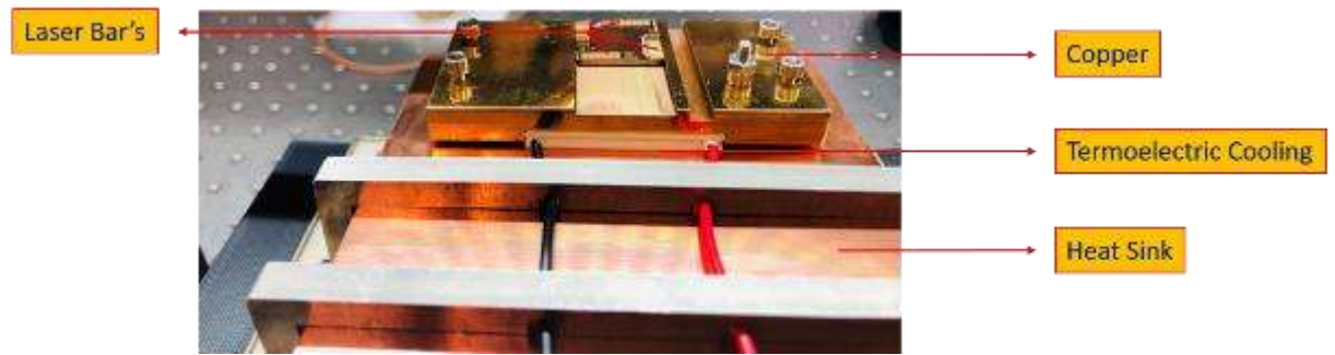
Figure 3-11. Closer look at the heat spreader elements
