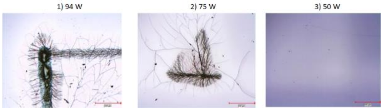
Figure 5-3. Optical microscope images produced after heat treatment with various laser powers on coated glass surfaces at a scanning speed of 5 mm/s and a distance of 20 mm.
