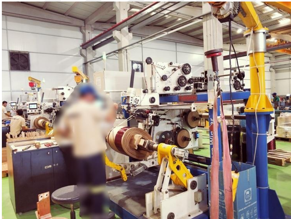
Figure 3.25. High-voltage winding production
