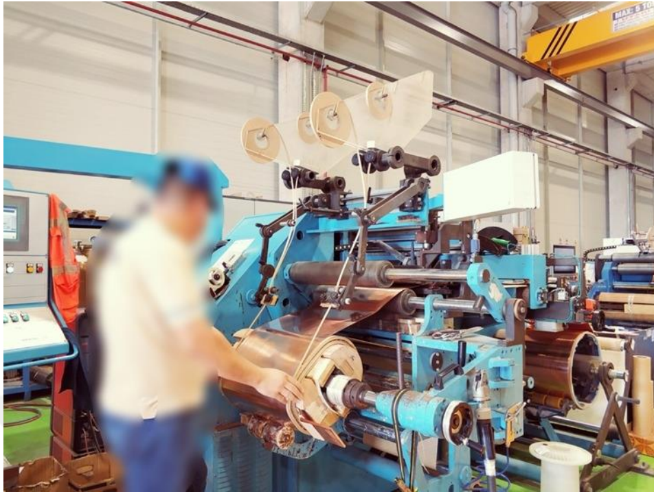
Figure 3.24. Low-voltage winding production
