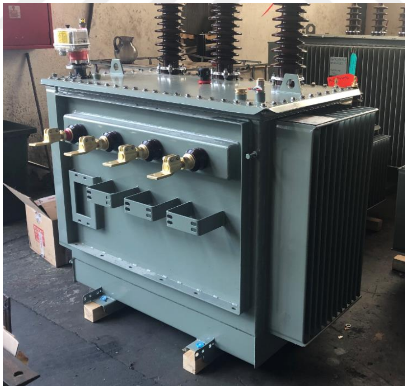
Figure 3.34. CSP transformer prototype (Front view)
