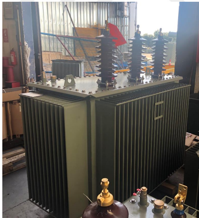
Figure 3.36. CSP transformer prototype (Rear view)
