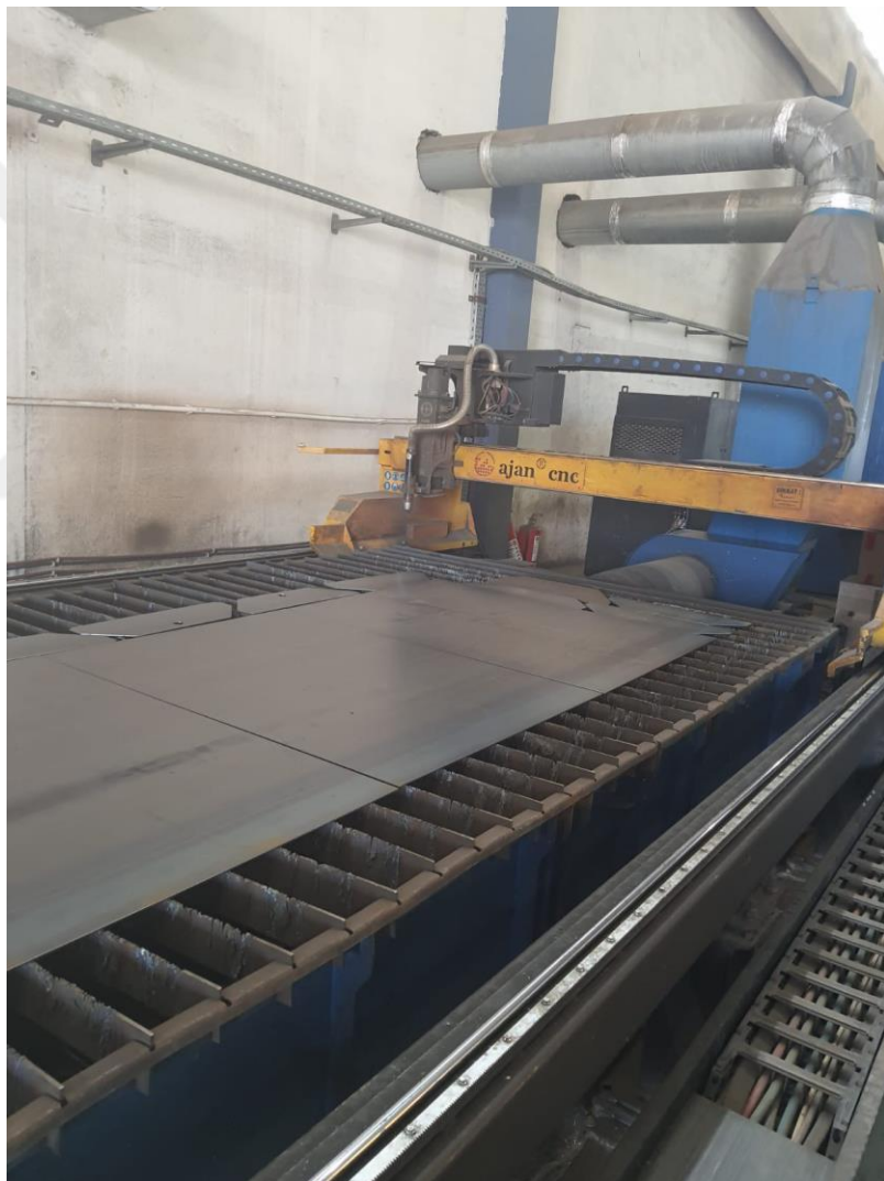
Figure 3.29. Tank base and carrier cutting stage
