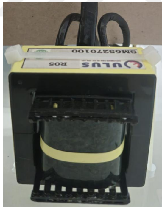
Figure 6.4. High frequency transformer used in the prototype
