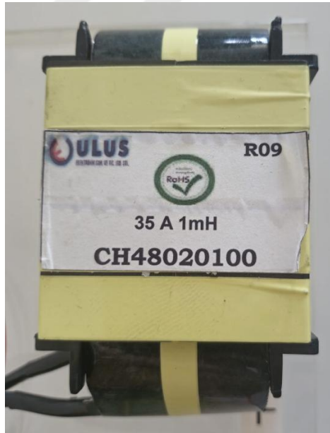
Figure 6.5. Boost converter inductor used in the prototype
