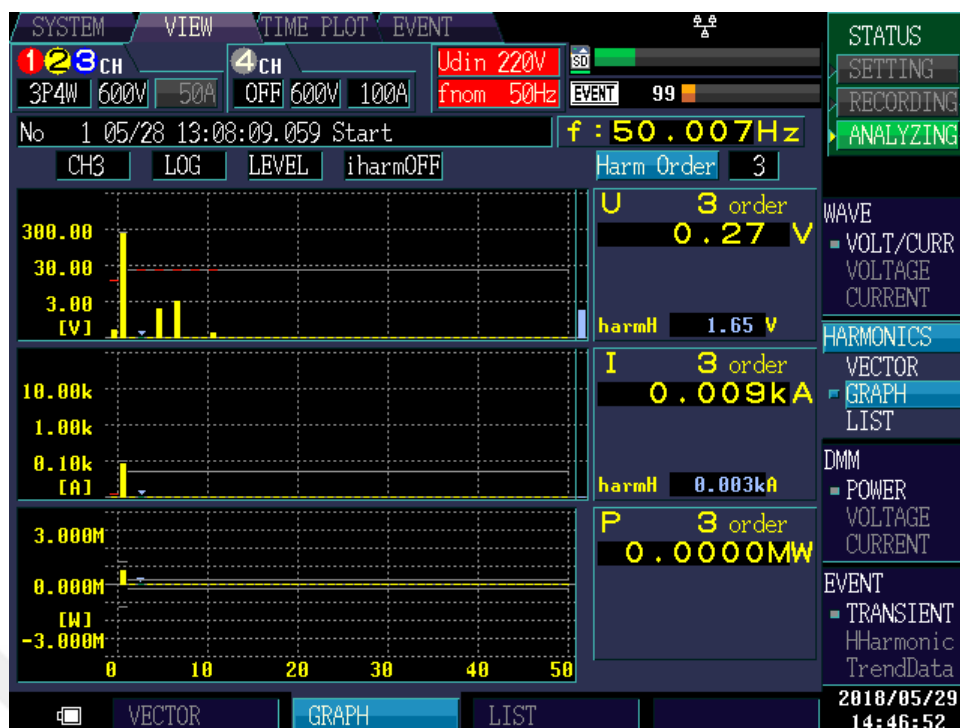
Figure 4.13 Phase C 3 rd harmonic Current Before Compensation
