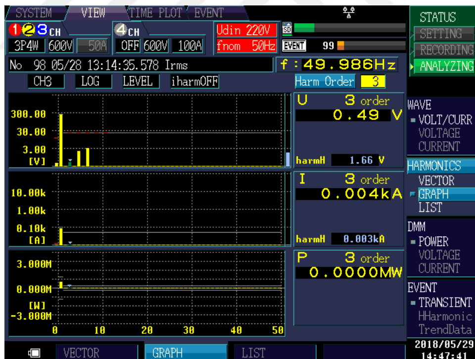
Figure 4.14 Phase C 3 rd harmonic Current After Compensation
