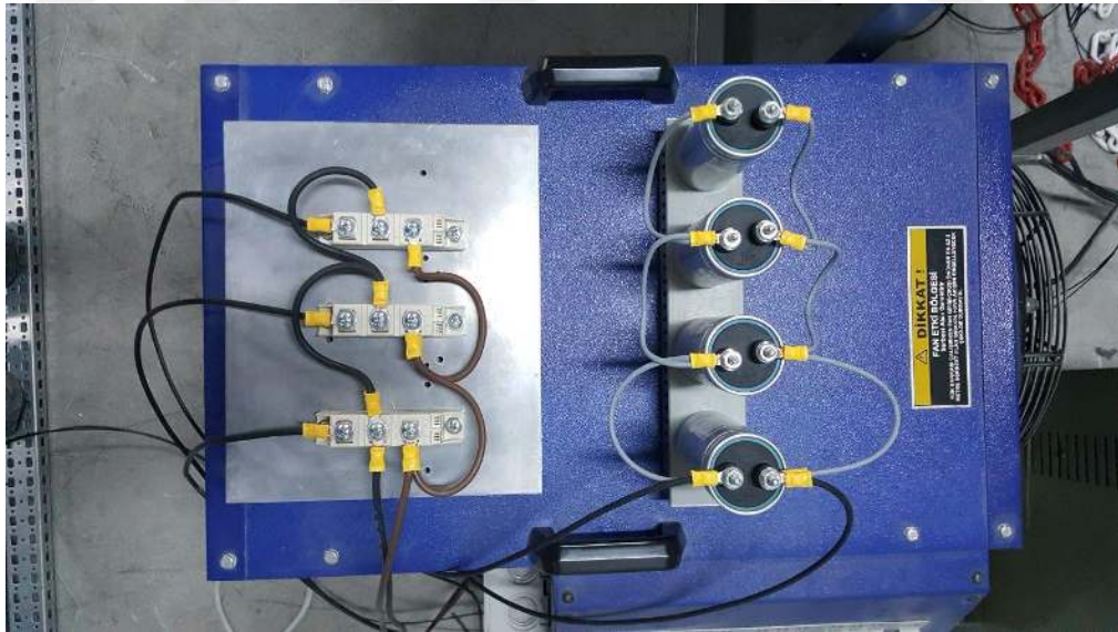
Figure 4.16 Three Phase Rectifier Implemented Circuit
