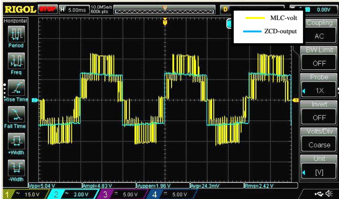
Figure 7.16 Multilevel inverter voltage and zero cross signal
