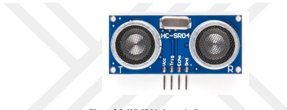
Figure 3.8. HC-SR04 ultrasonic distance sensor
