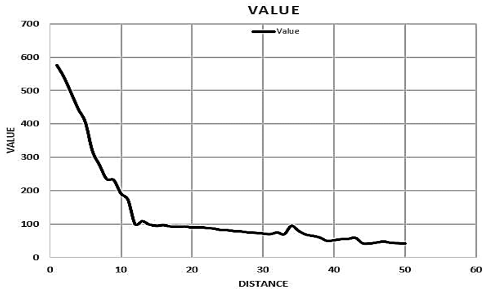
Figure 2.15: Flame sensor analogue output voltage against distance.
