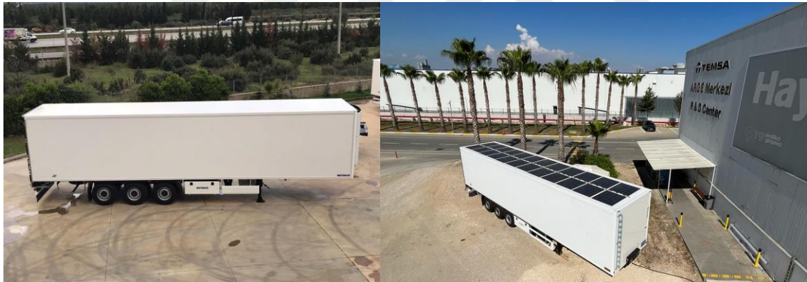
Figure 3.24. Before And After The Solar Panels Installation.
