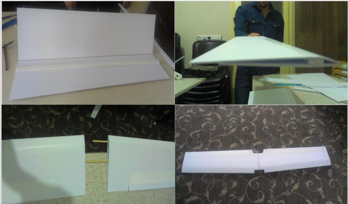
Fig. 6.4 Construction procedure of the wing
