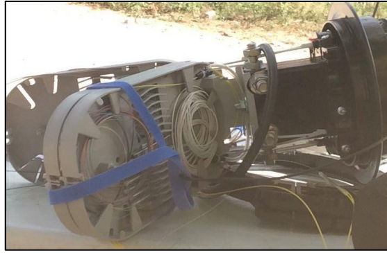
Figure 3.29: Optical Distribution Box (ODC).
