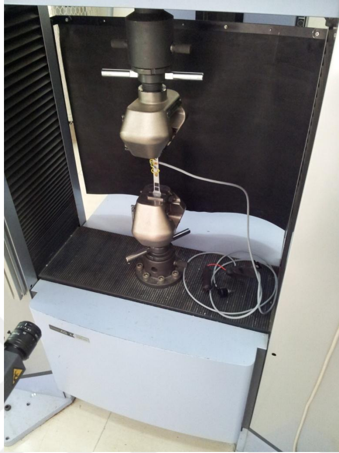
Figure 5.1 Universal testing machine and telemetry setup
