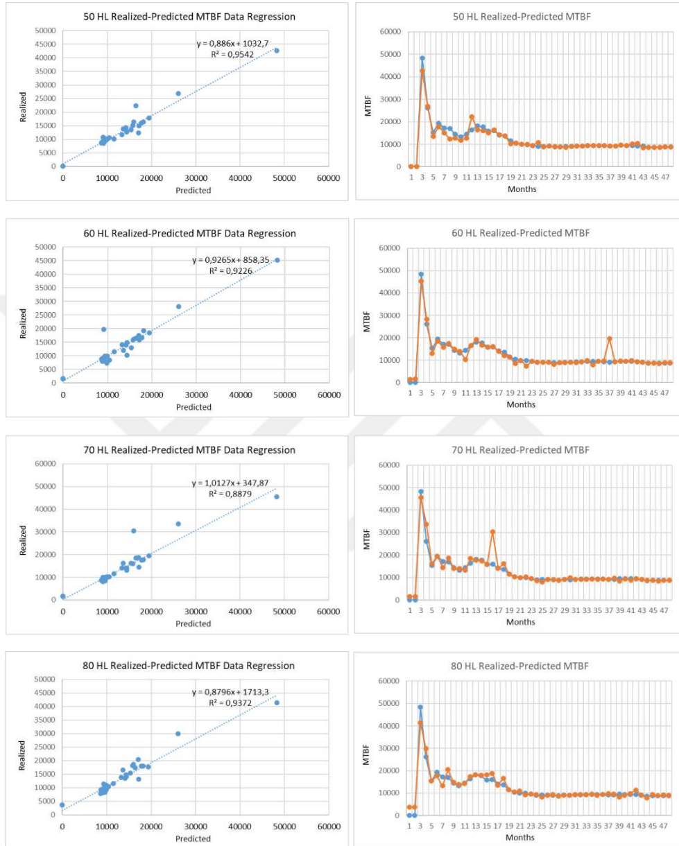
Figure 4.10. Structured ANNs Performances from 50 to 80 HL (Yellow Series: Predicted Data, Blue Series: Realized Data)
