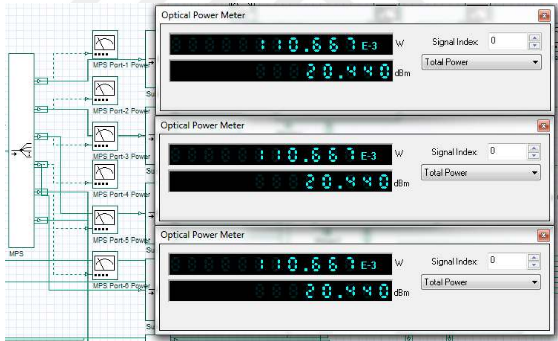
Figure 4.5 Output power measurements of 1st, 3rd, and 5th ports of the MPS power splitter
