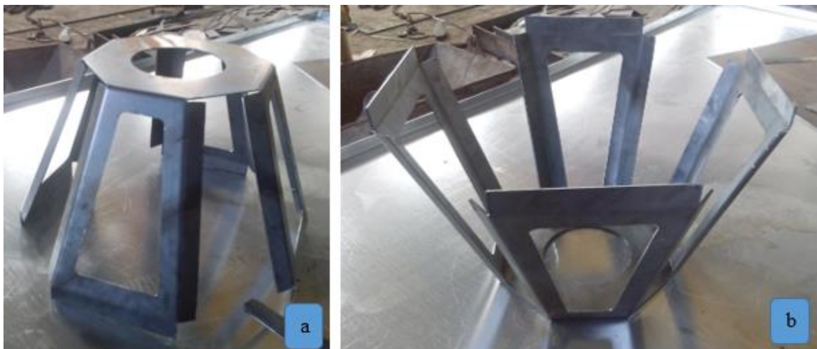
Figure 3.32 Largest part from base body after folded the wings.
