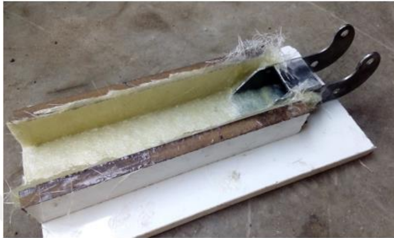
Figure 3.46 Upper arm working to fiberglass.
