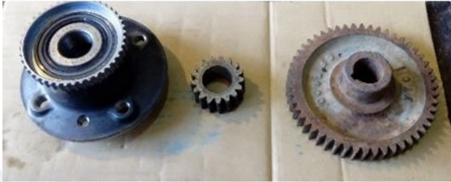
Figure 3.41 Rotary joint parts before machining.
