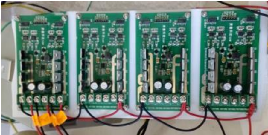
Figure 4.7 Dual 15A H-Bridge DC Motor Drivers installed on plastic board.
