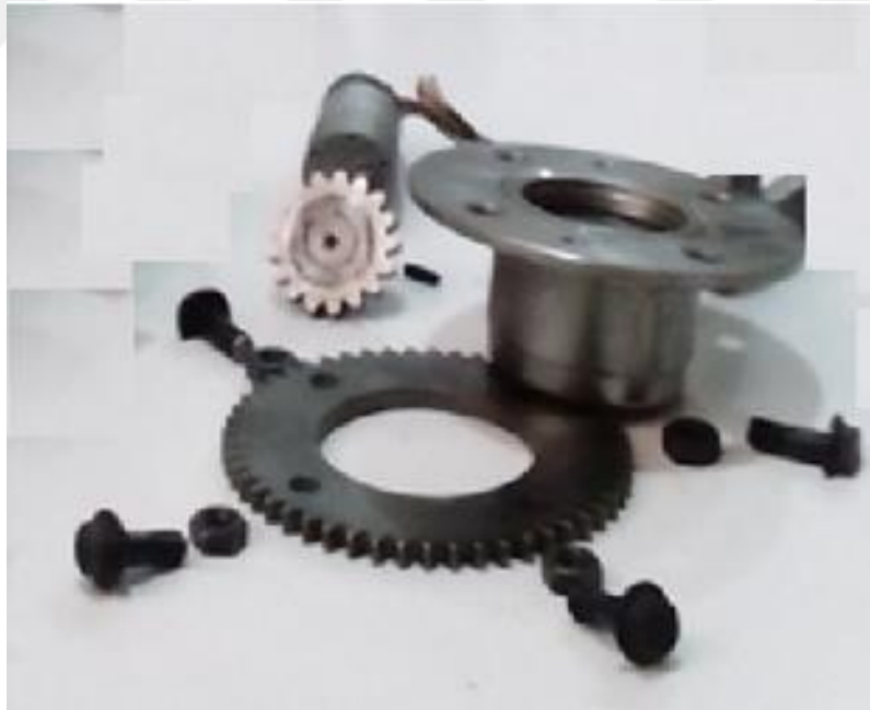
Figure 3.42: rotary joint parts after machining.
