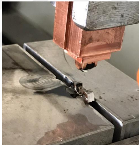
Figure 6.18 The EDM process for the secondary middle part.
