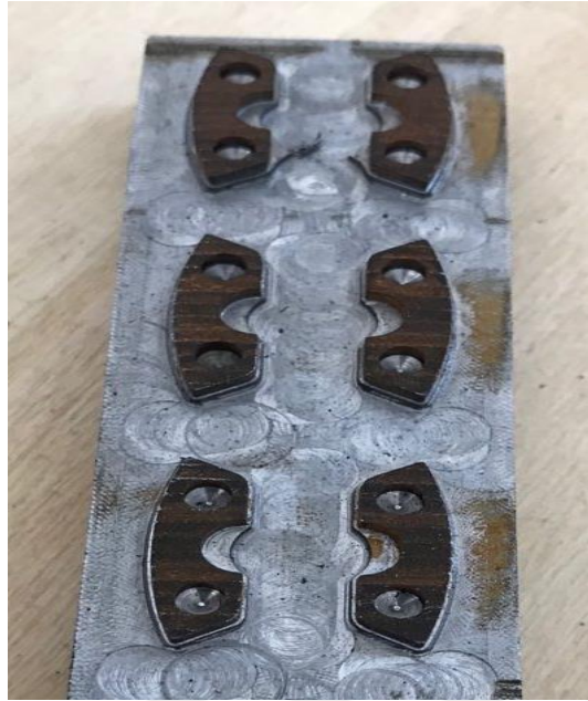
Figure 6.17 Original bulk after the wire cutting process.
