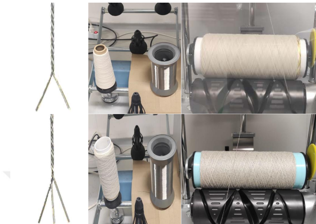
Figure 5.4. Double and triple twisting processes of conductive yarn and wool yarns
