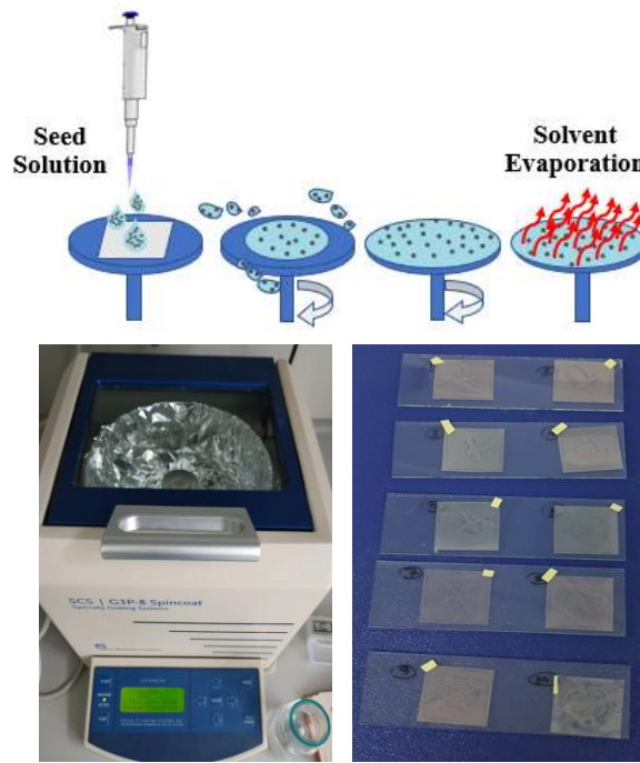
Figure 2.3. Illustration of spin coating process, photographs of spin coater, and seed layer coated ITO/PET substrates
