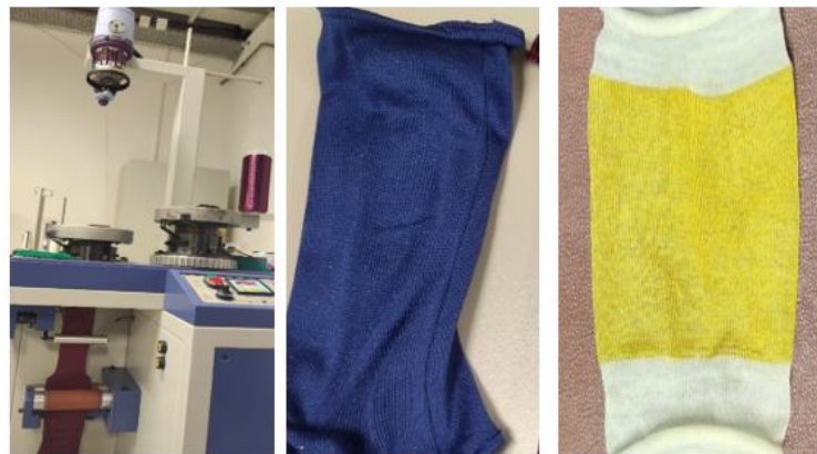
Figure 5.8. Non-conductive (blue) and conductive (yellow) fabrics obtained with a circular knitting machine
