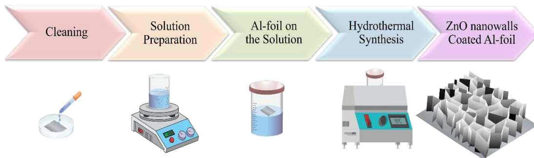
Figure 4.2. Schematic illustration of hydrothermal synthesis of doped ZnO nanowall arrays on Al-foil
