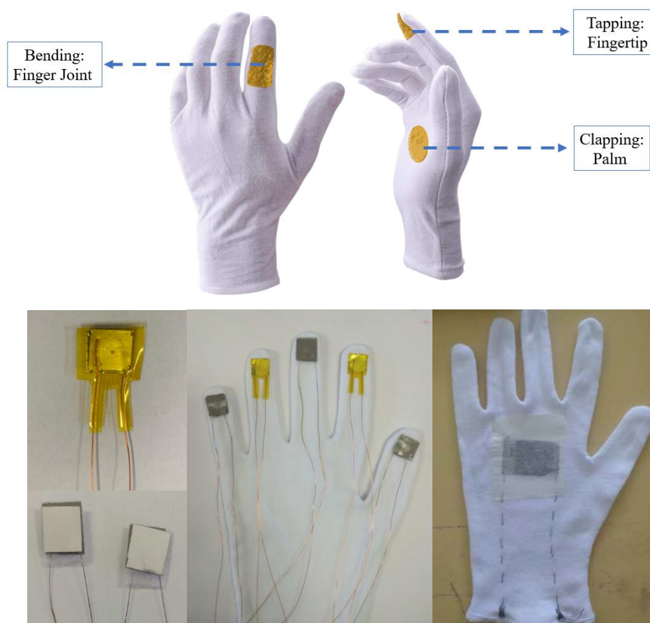
Figure 5.10. Integration of ZnO nanowall-based nanogenerator modules into gloves
