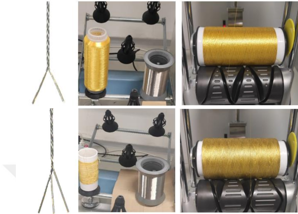
Figure 5.7. Double and triple twisting processes of conductive yarn and yellow polyester yarns
