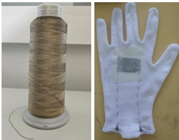
Figure 5.35. Photos of the silver-coated polyamide conductive thread and the module integrated into the palm of the glove with the silver-coated polyamide conductive thread
