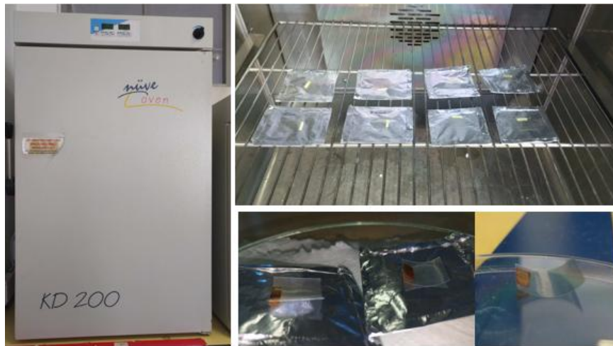
Figure 2.4. Oxidation process applied to seed layer deposited ITO/PET substrates at 200°C for 3 h
