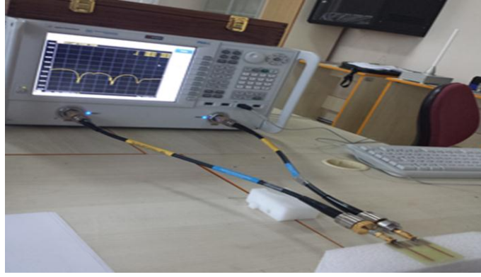
Figure 4.58 Measurement setup for the fabricated antenna system.
