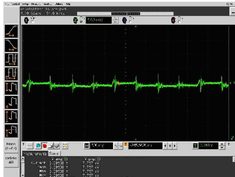
Figure 5.38 Output voltage ripple waveform at full load.
