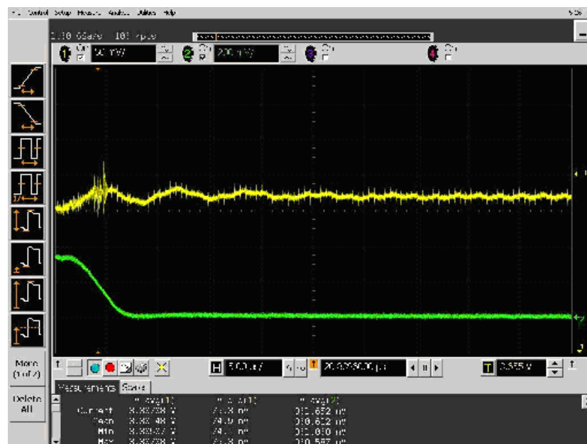
Figure 5.49 Output voltage transient overshoot (30 A to 0 A).
