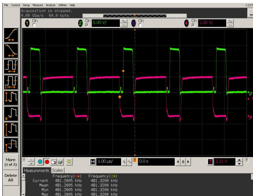
Figure 5.36 High side MOSFET and low side MOSFET PWM signals of fourth phase.
