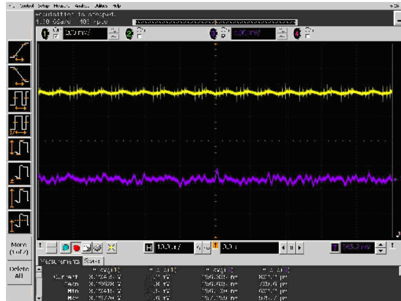
Figure 5.19 Output voltage ripple waveform.
