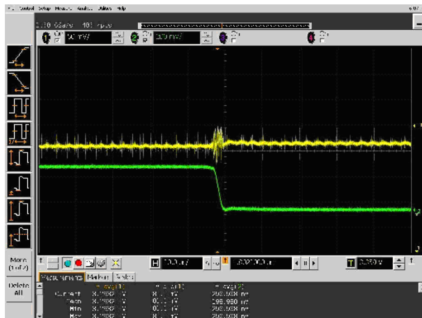
Figure 5.30 Output voltage transient overshoot (30 A to 0 A).
