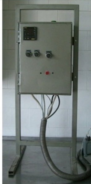
Figure 3.3: (a) Microwave and conventional system combined oven b) Control panel
