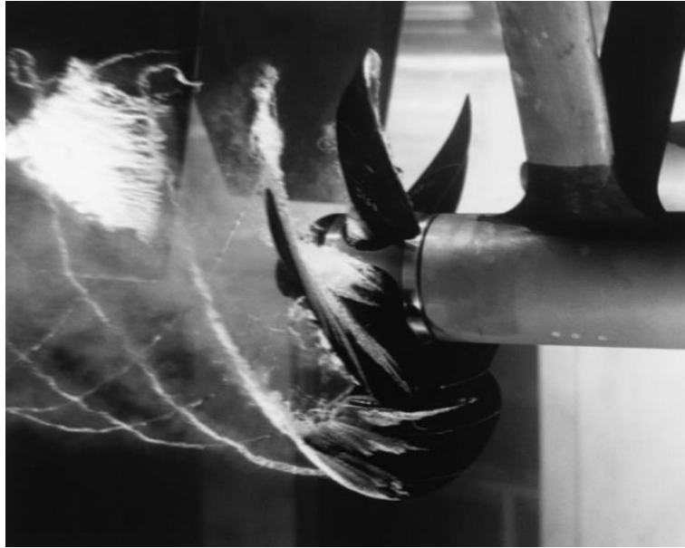
Figure 4.9 Cavitation of propeller ( http://www.dt.navy.mil )
