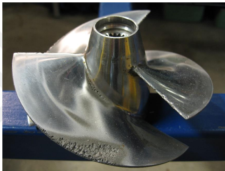
Figure 4.8 A propeller which is damaged by cavitation (Common license, 2006)
