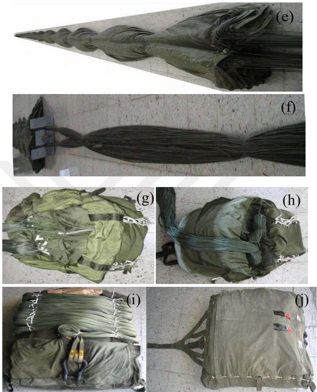
Figure 2.4 (continued): Preparation of cargo parachute, (e) Tying canopy, (f) Tying suspension lines (g) Stowing the canopy in deployment bag, (h) suspension lines tied on retaining strap loops, (i) Suspension line stowage completed, (j) Packing completed
