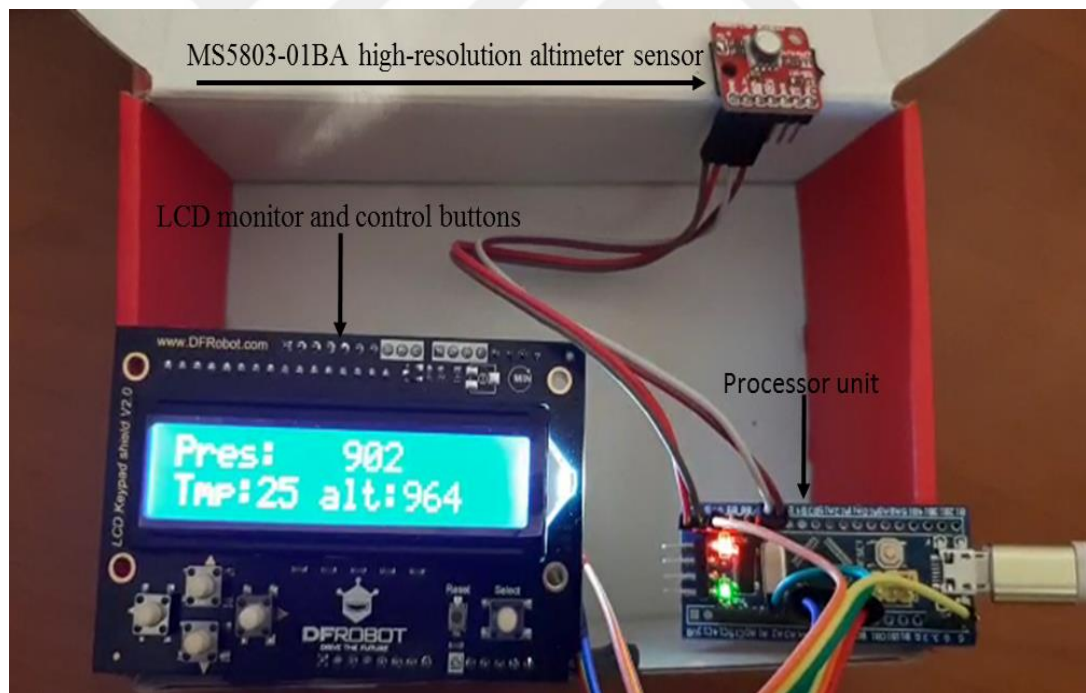
Figure 3.5 MS5803-01BA high-resolution altimeter sensor
