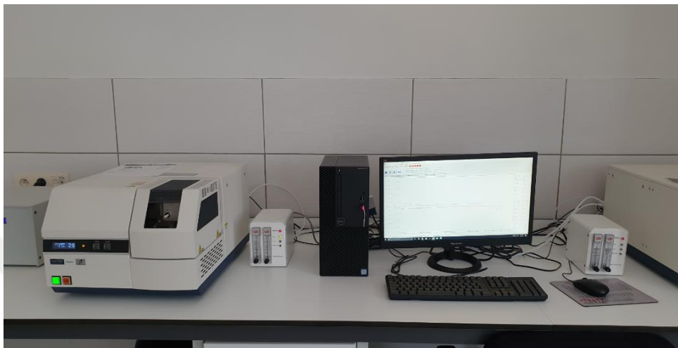
Figure 3.10 Hitachi STA 7300 TGA / DTG device.
