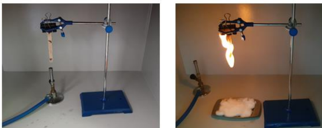
Figure 4.20 Vertical fire test setup and reference sample.
