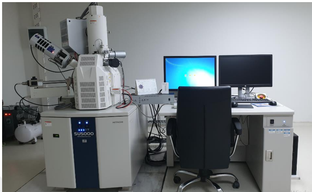
Figure 3.8 Hitachi SU5000 Scanning Electron Microscope.
