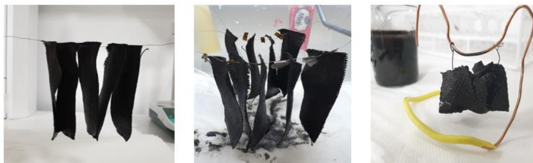
Figure 3.4 PDA coated flax fibres.
