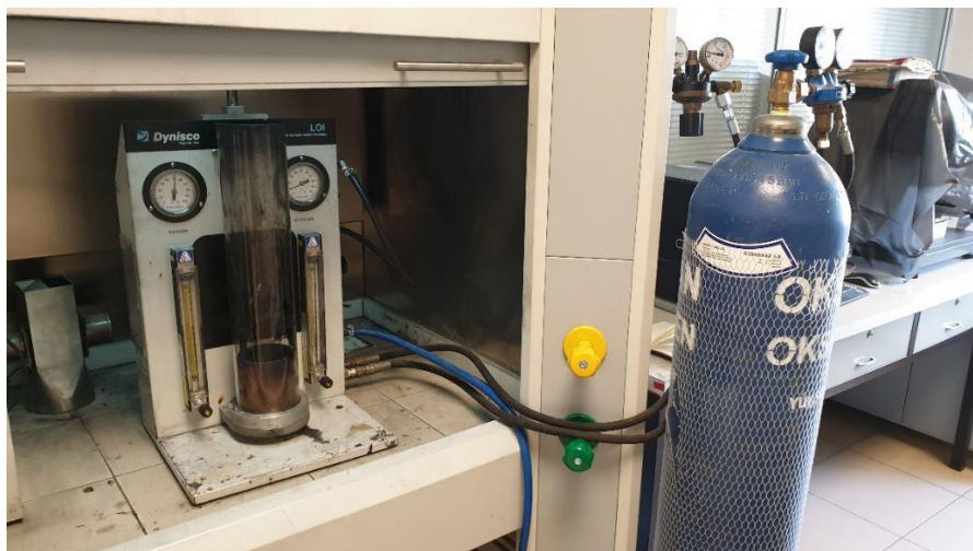
Figure 3.11 LOI test device.
