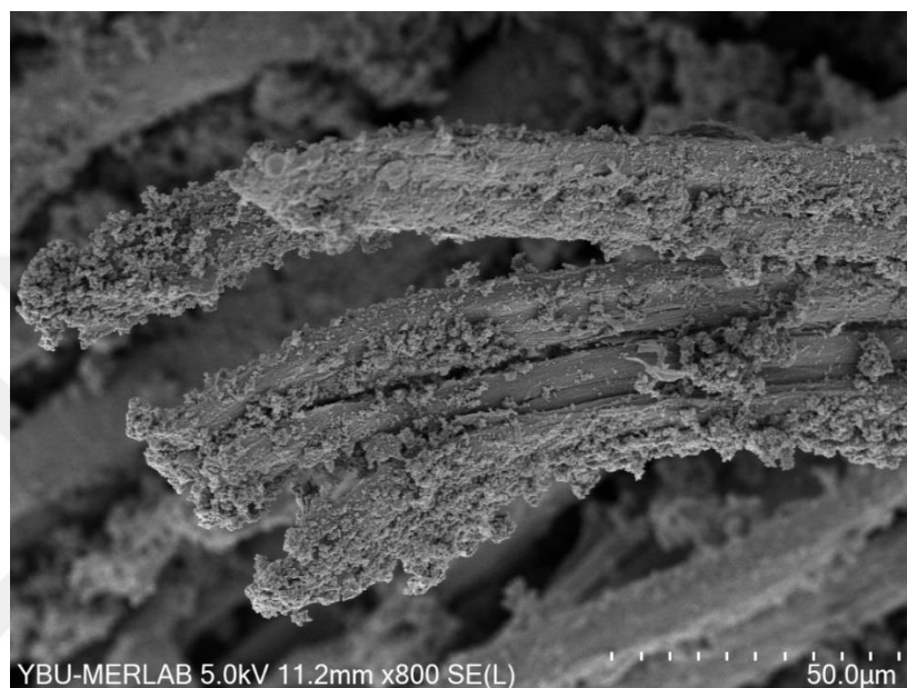
Figure 4.2 Flax fibre surface coated with PDA.
