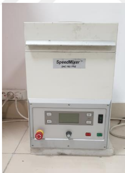
Figure 3.6 Speed Mixer dual asymmetric centrifuge device.
