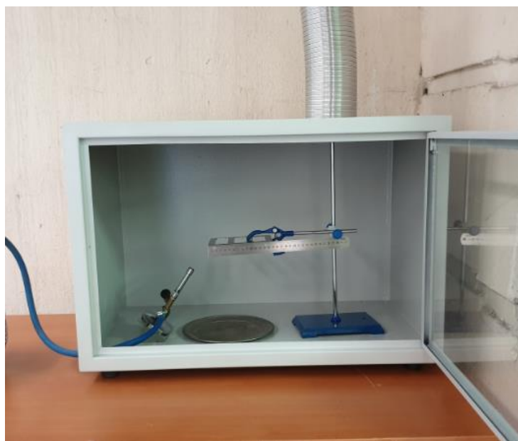
Figure 3.12 UL-94 test device.
