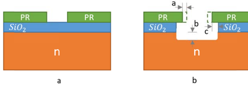
Figure 6.5 (a) A structure ready for etching and (b) result of etching
