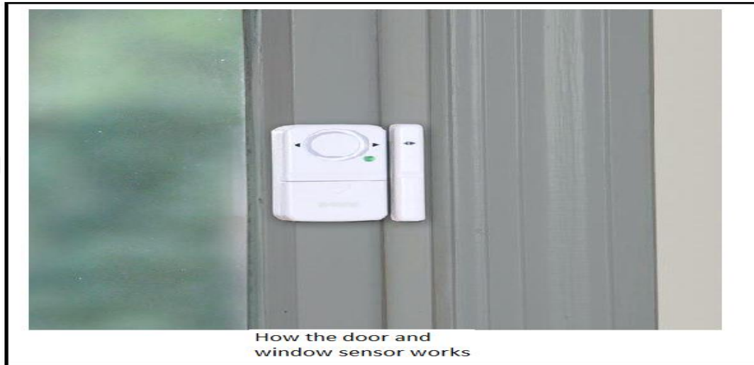
Fig. 1.7: How the door and window sensor work [21].
