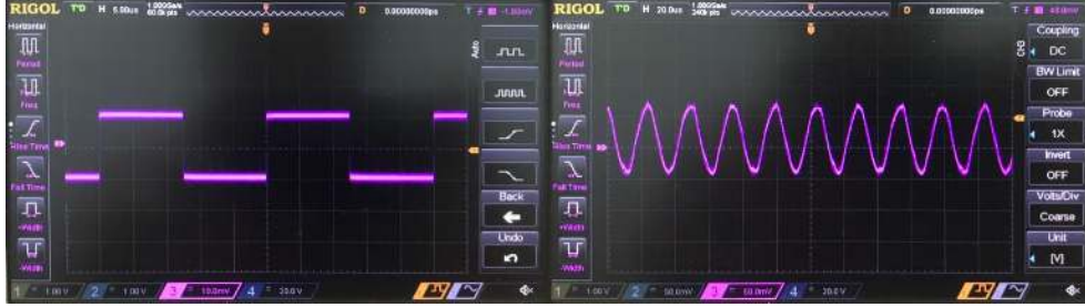
Figure 3.3. The square wave (left) fed to the transmitter transducer and the sine wave (right) emanating from the narrow-band filtered and amplified circuit of the sensed signal.
