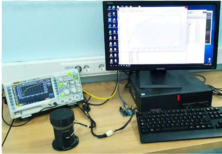
Figure 5.2. Oscilloscope and computer supported experimental setup.
