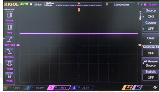
Figure 3.5. Output of the sine signal after the signal is passed through envelope detector.
