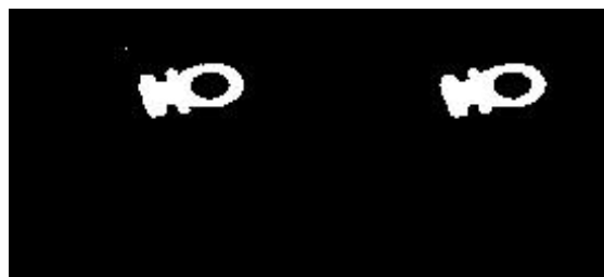
Figure 6.7. Applying the median filter removes the noise
