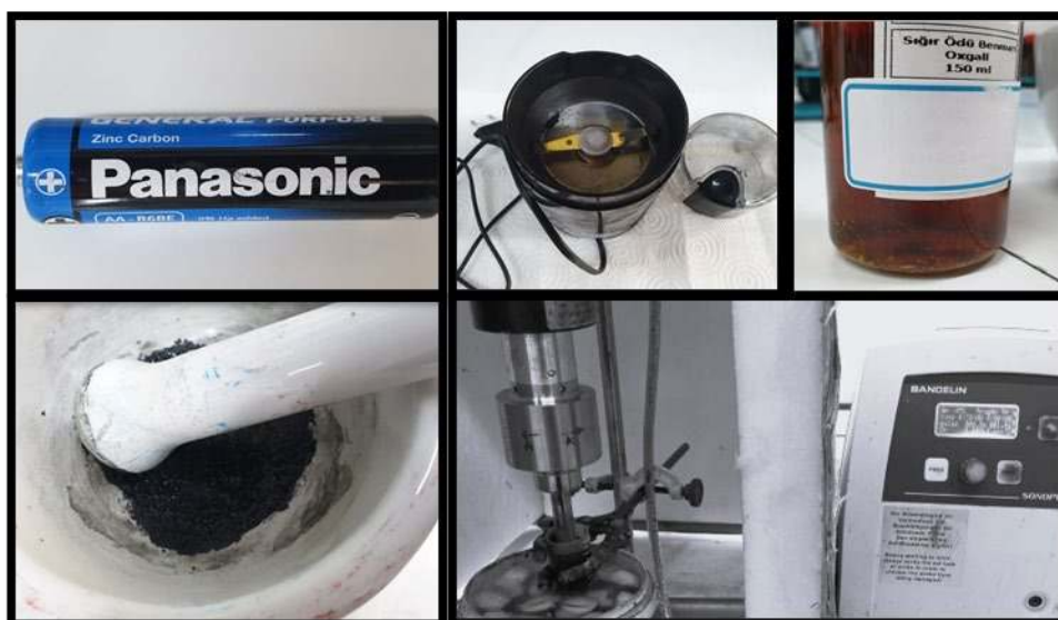
Figure 2.2 : Ink preparation steps for CWM a) Spent zinc carbon battery b) coffee grinder to turn into powder form c) oxgall d) mortar and pestle to grind the cathode powder e) sonication process.
