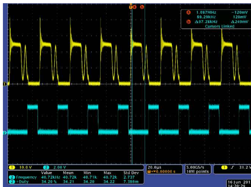
Figure 4.28 A sample SMPS is made and tested with SMPS transformer test device – PWM Gate Drive signals at steady state with 3.3V output and 0,6 A load.
