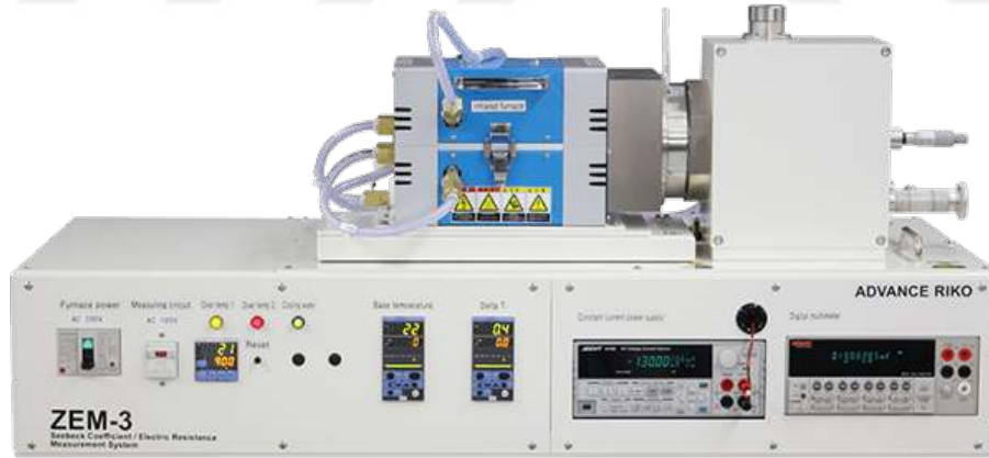
Figure 4. 8 Electrical resistivity and Seebeck coefficient measurement system.
