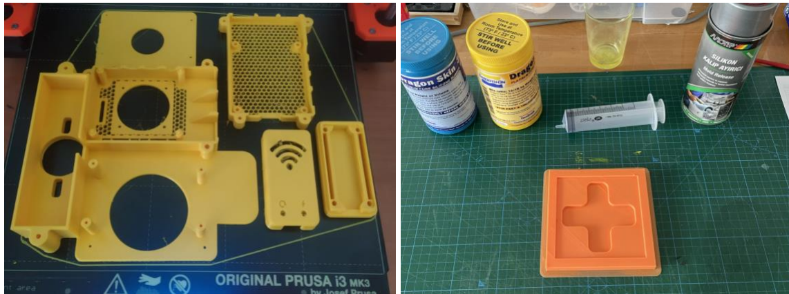
Figure 16 a) 3D Printed casing for the electronics, b) The mold for plus-shaped surface
