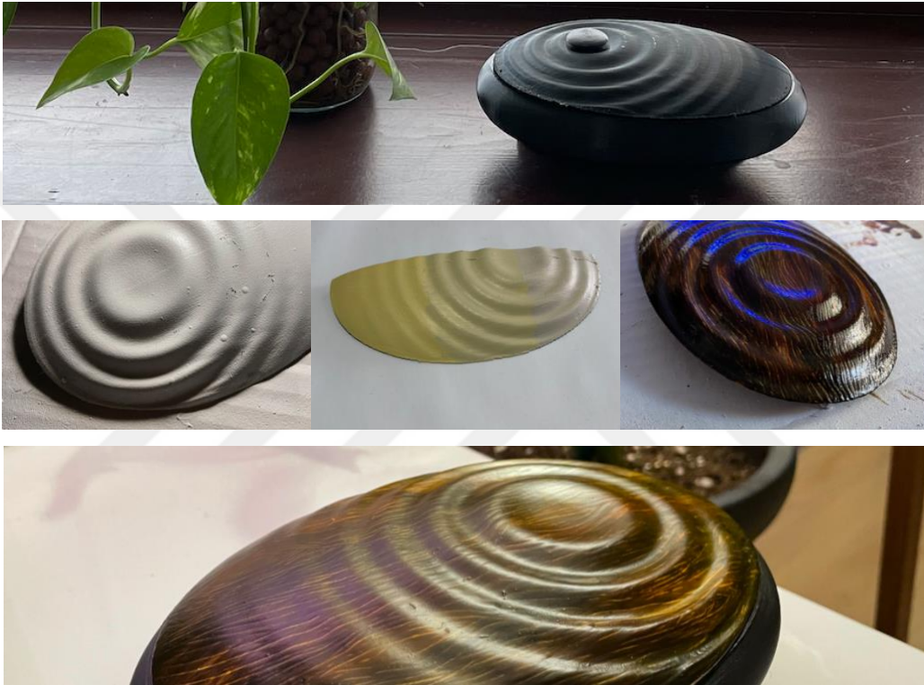
Figure 11 Final Painting Process a) 3D Prints, b) Primed, c) Sanded, d) Aged, e) Final
