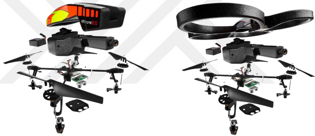
Figure 3.1 Parrot AR Drone quadrotor disassembled view (Piskorski, 2010)
