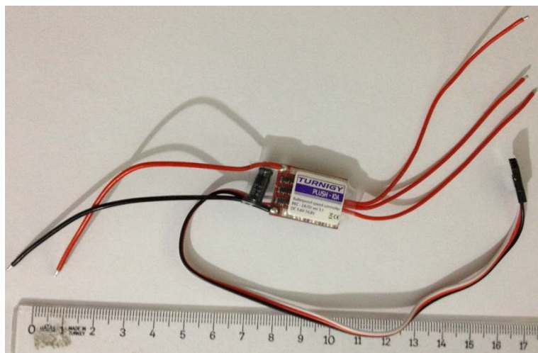
Figure 2.9 Turnigy Plush 10A Programmable ESC with BEC (Personal archive, 2017)
