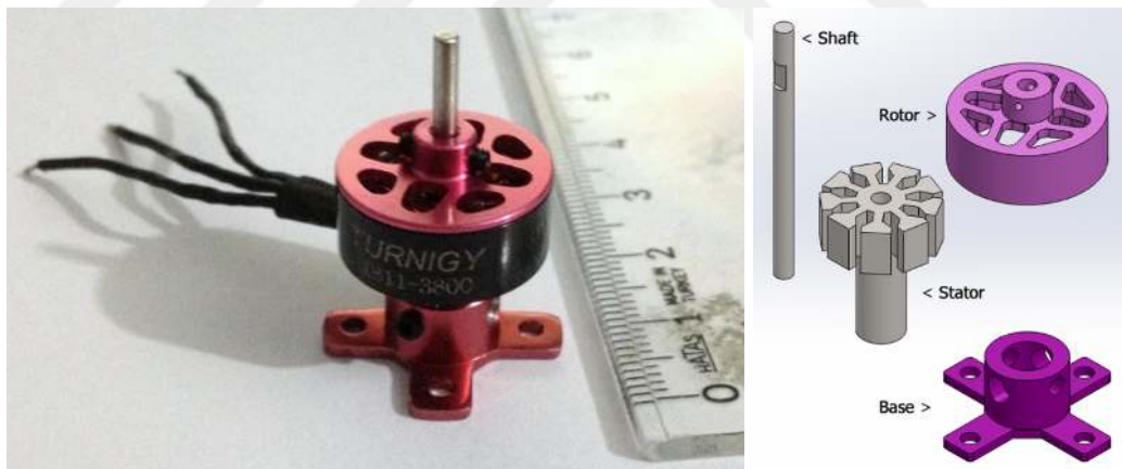
Figure 2.7 Turnigy 1811 brushless DC motor and exploded 3D drawings (Personal archive, 2017)
