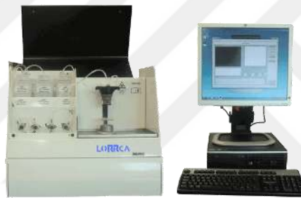
Figure 2.8 LORRCA MaxSis (the laser-assisted optical rotational cell analyzer, Mechatronics, Netherlands (Hardeman et al., 1994).
