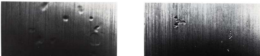
Figure 2.8 Indentation due to hard particles (FAG, 1985).
