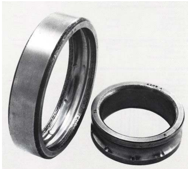
Figure 2.7 Indentation of soft particles (FAG, 1985).
