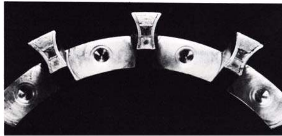
Figure 2.27 Cage fracture due to vibration (FAG, 1985).
