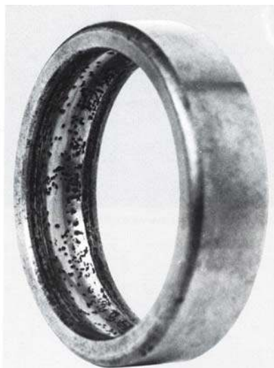
Figure 2.10 Corrosion due to rust (FAG, 1985).
