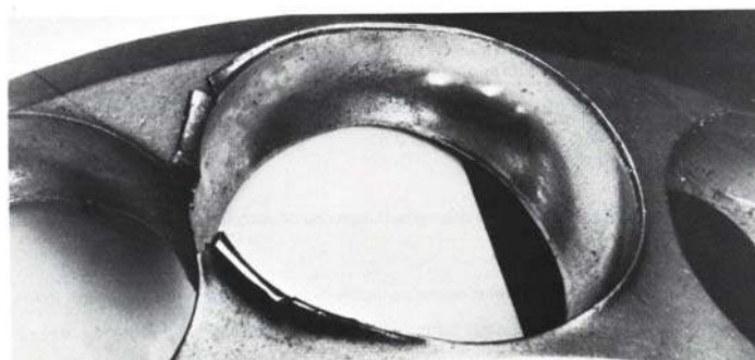
Figure 2.28 Cage fracture due to misalignment (FAG, 1985).
