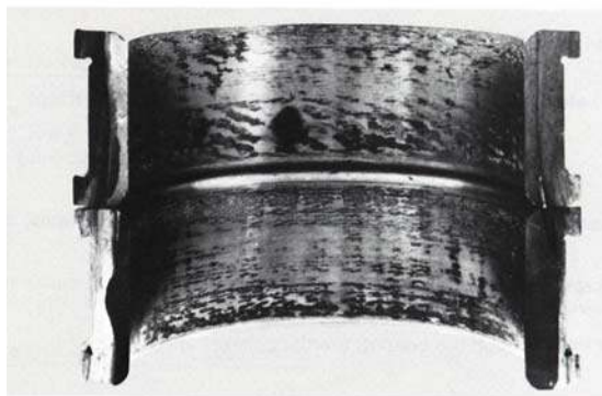
Figure 2.12 Fretting corrosion (FAG, 1985).
